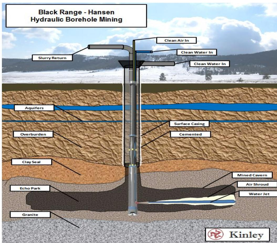
Once a borehole has been completely mined, the remaining cavity will be filled with specialized cement slurry. The borehole is then backfilled and the top of the casing is plugged with bentonite and cement before final completion with a soil cap.
