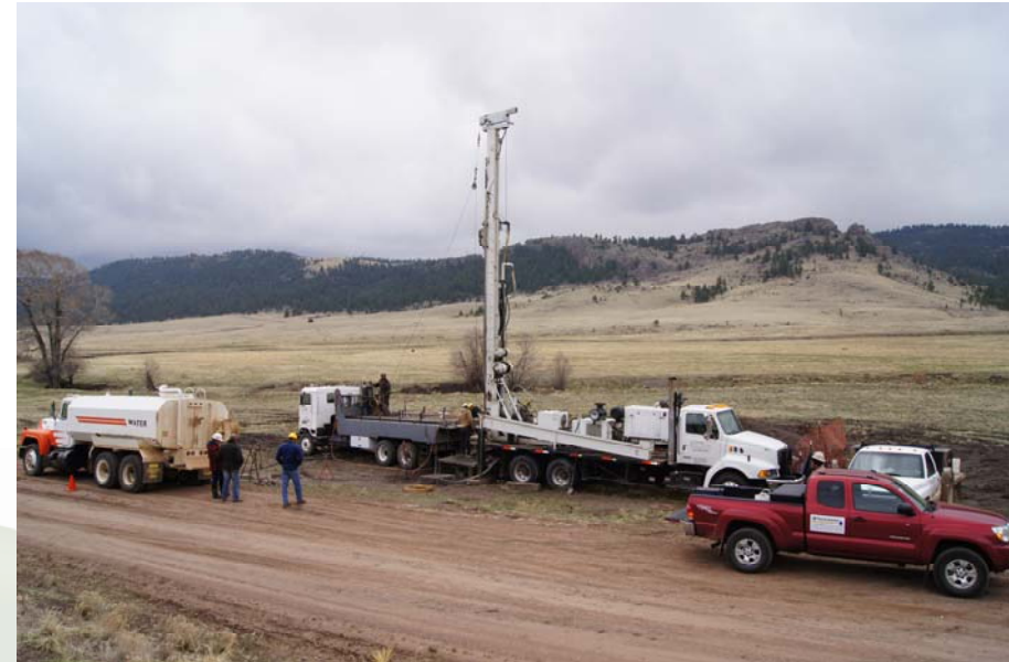
Diamond core drilling at the Hansen Uranium Deposit.
