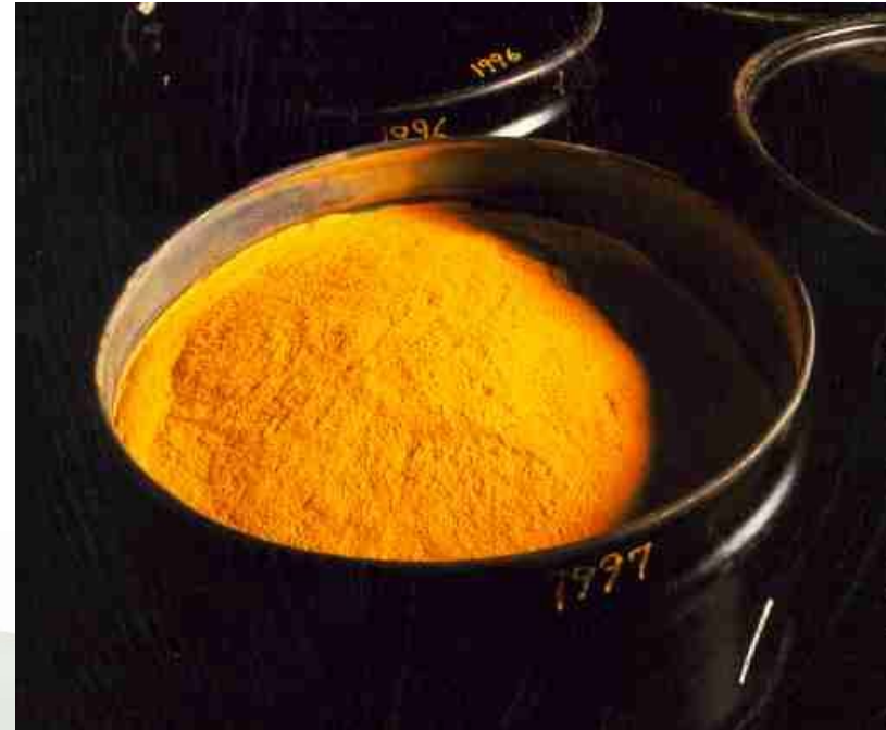
Yellowcake – typically the first stage product recovered when processing uranium ore.
